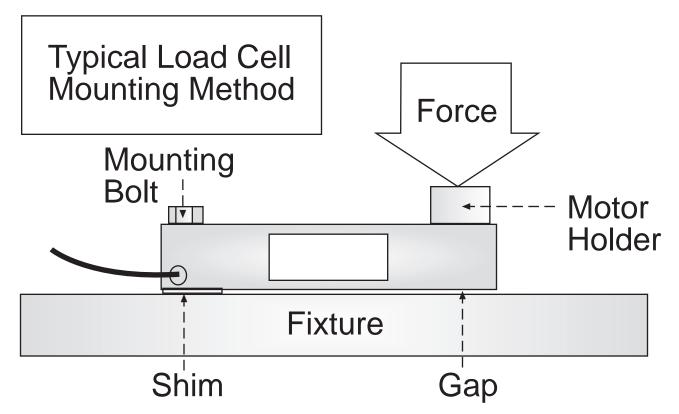
The load cell is a precision piece of hardware and should be handled accordingly. Protect the white silicone covering on the flat side of the load cell as this covers the bridge resistor elements that are bonded to the metal. Typically load cells only flex a couple of thousandths of an inch so size the shim accordingly - 5 thousandths is often too much and will allow the cell to exceed its safe overload. Test with weights to determine you have the proper amount of deflection.
